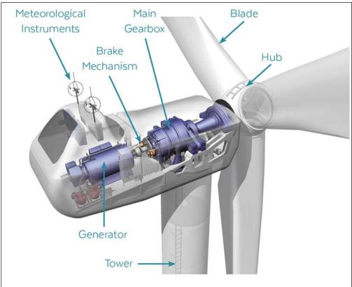
Figure 4-3 Turbine nacelle and-5 hub components
