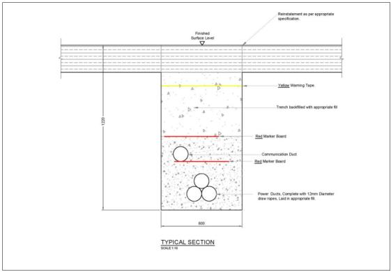
Figure 4-9 Typical Cable trench cross section detail
