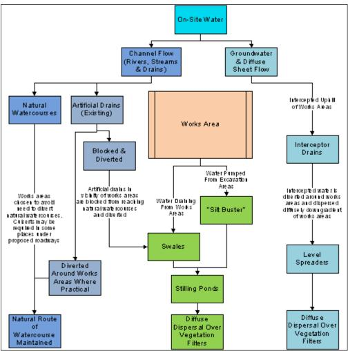
Figure 4-16 Proposed Development Drainage Process Flow
